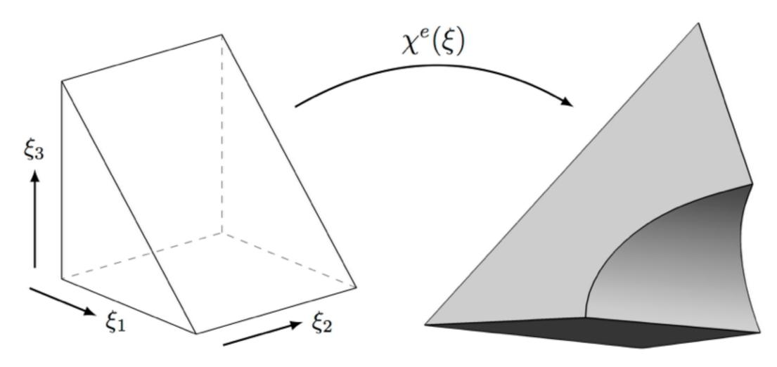
Shape function is a mapping from reference element (parametric coordinates) to mesh element (physical coordinates)
