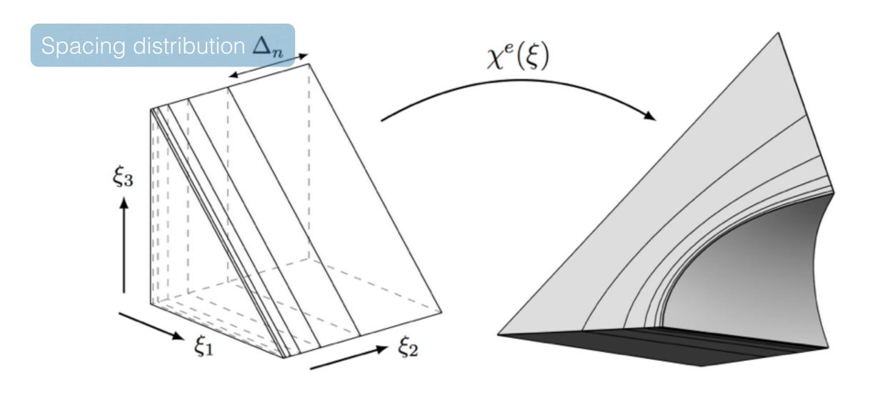
Subdivide the reference element in order to obtain a boundary layer mesh
